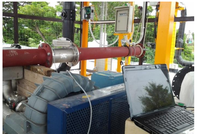
Oscillating Flow Meter for bio gas, with flow computer
