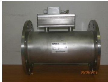
Oscillating Flow Meter for bio gas, with flow computer
